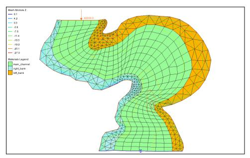
Figure 2 Mesh with Materials turned on in the Display Options dialog
