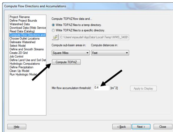
3. Click on the “*Compute Topaz*” button which will compute the flow directions and accumulations and infer the streams based on DEM data. Click on “*Close*” after computations are complete. Move the modeling wizard dialog to the side of the WMS window to see blue lines added to the display that represent areas of high flow accumulation.
